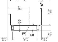
EI Electrical inlet (power) = EQ = Equipotential screw
